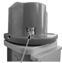
EXH : Air being exhausted
