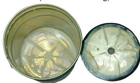
Pail and follower plate (Grease remaining)
